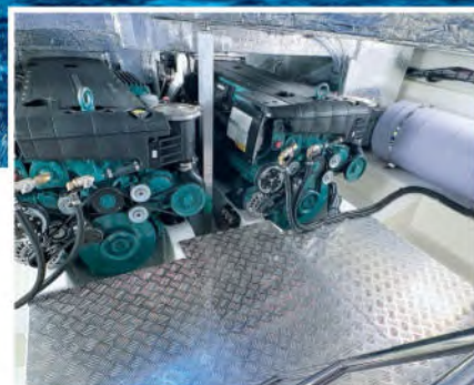
ABOVE: There's masses of space ahead of the stern-drive rig for a gyro and a generator
