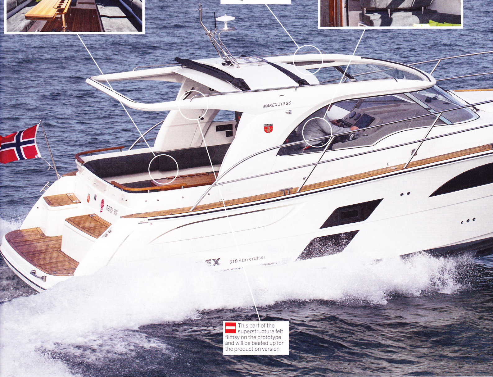
One major change for the production run will be stopping the lip on the sunroof from impacting standing headroom
